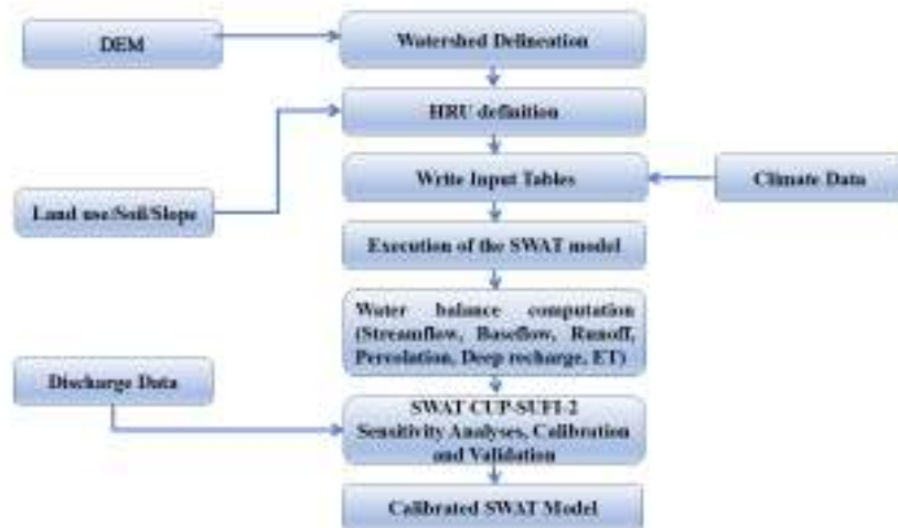
Figure 9: Flowchart of the SWAT Processing Steps for the CGRB
